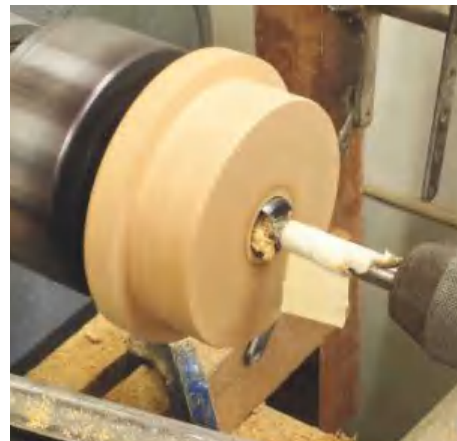
▲ Pic.12 The hole for the stem is drilled on the lathe and the masking tape is used as a rough depth guide. A 25mm hole seemed to be about the right size, but as you will see later, if you go too big then this will cause some problems
